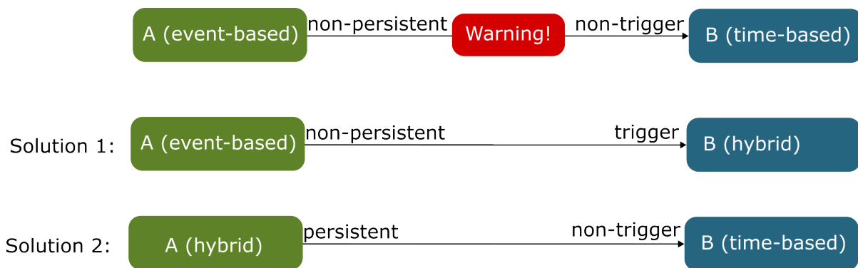
Fig. 1: A non-persistent output connected to a non-trigger input leads to a warning.
